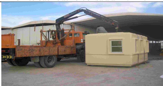
3.2M long Cabin being lifted for transport
